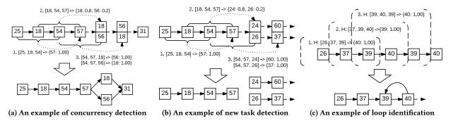
Figure 4: Examples of using LSTM for task separation and workflow construction.
