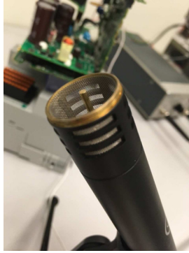
Figure 6: AKG P170 condenser microphone without transducer serving as an electromagnetic probe.
